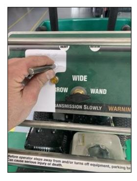
Using a step-drill, drill hole to ½" diameter and install toggle switch with notch positioned as shown.
