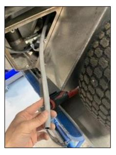
Run hose through the bottom of the nose cone and pull hose out (approx. 3") through the open hole in the RH bumper support.
