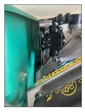
Use the 1/4-20 bolts & nuts and 1/4" flat washers provided to fasten the pump mounting plate to the existing holes in the hood.
