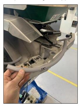
Route the 14" hose along the inside surface of front bumper as shown below (image includes installed auxiliary nozzle)
