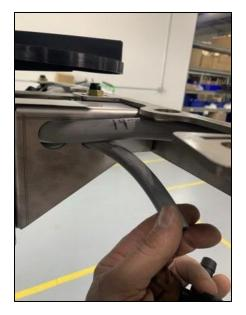
**NOTE:** On older units, the RH bumper support my not include the extra hole for routing the supply line through. In this case, use a step drill to drill a 3/4" hole adjacent to the existing hole or contact Turfware for a replacement bumper support.
