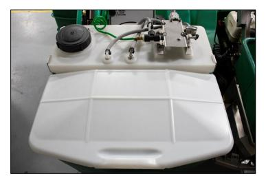
Final assembly showing installed spot-sprayer with slide-on cover.
