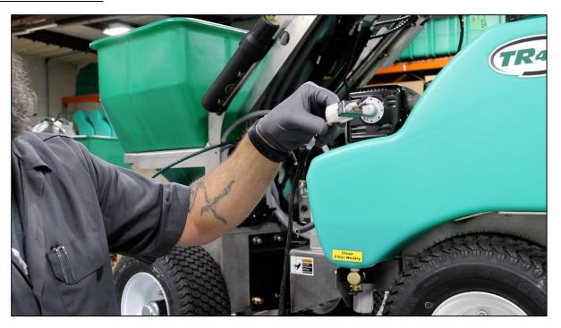
Remove the plastic plug in the dashboard and install the Toggle Switch supplied with the wiring harness.
