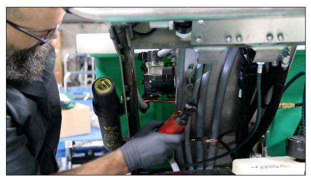
After tank clip installation, fully tighten the Support Bracket bolts using 7/16" wrench and socket. Double-check to ensure tank is securely mounted to hopper.
