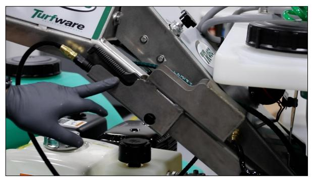
Using the original hardware from the single holster, install the double wand holster supplied with the kit in the same location as the original holster.
