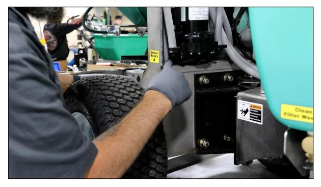
Continue to feed the hose down through the hole in the far-left side of the lower front deck adjacent to the main spray pump.
