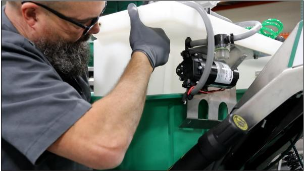
The Spot Spray Tank mounts over the rear wall of the hopper. When sliding the tank in place, make sure the rear wall of the hopper is between the Spot Spray Tank and the Tank Support / Pump Mount bracket (see above).
