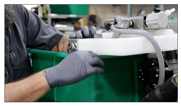
Push the Spot Spray Tank firmly into the rear wall of the hopper and tighten brackets with 1/2" wrench.
