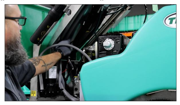
Feed the harness through the opening in the back of the dashboard and route it along the existing wiring harness; zip-tie in place.
