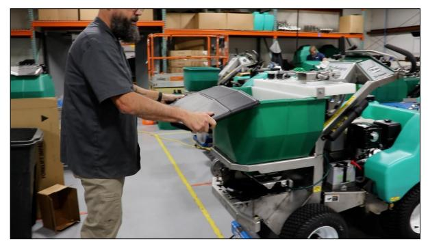
Slide the half hopper lid supplied in the kit over the front of the hopper. The lid will snap into place when properly seated on the hopper against the Spot Spray Tank.
