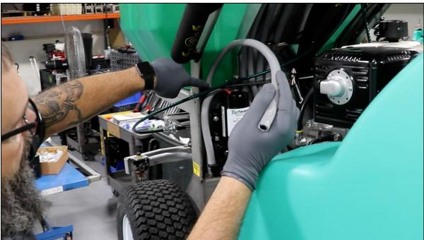
Route the hose down through the hole on the far-left side of the firewall.
