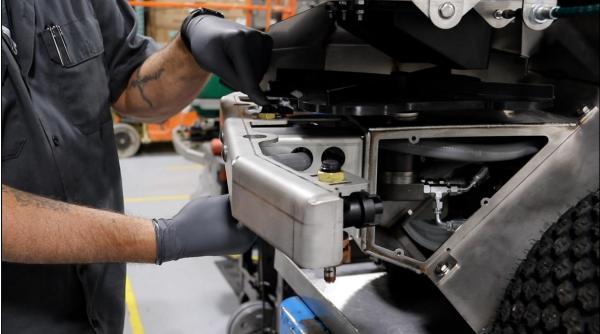
Feed the hose (shown in blue) up over the top of the front axle and into the nose cone area. Connect it to the reducer on the end of the installed spot spray nozzle.
