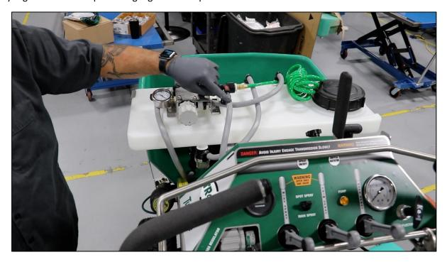
Turn the shut-off valve on the regulator to the "open" position (handle facing toward the hose); liquid should be dispersed from the Spot Spray Tank via the auxiliary nozzle mounted on the spray bar for the spot spray system.
